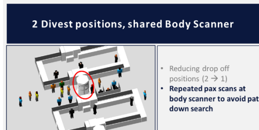
Figure 41: Lane with 2 divest pos. and shared Body Scanner
